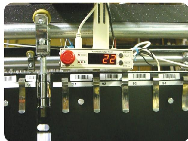
**AssembleMax:** Interfaced with the Railex garment sorting conveyor; current status with voice guidance in English or Spanish.
