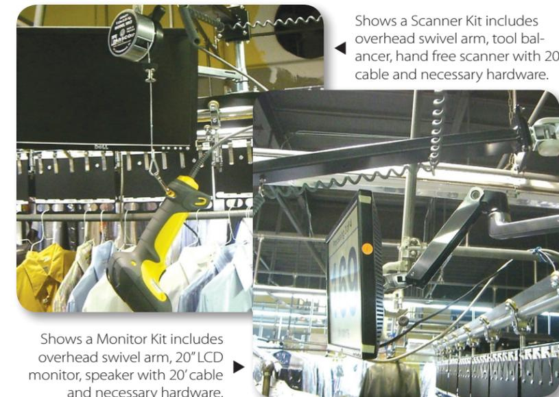
Shows a Scanner Kit includes overhead swivel arm, tool balancer, hand free scanner with 20' cable and necessary hardware.
