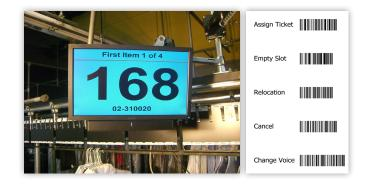
**Automatic Slot Extension:** The default settings allocate a maximum number of garments per slot. For example if this number was 4 or 5, the system would occupy that number of slots automatically dependent upon the number of garments in a given ticket item. For example, a ticket with 10 pieces will occupy 2 slots if the maximum slot setting was 5. However, the system will not designate the second slot until the first 5 pieces in the ticket has been completely transferred into the first slot.
