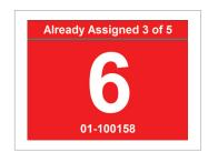
confirmation purposes. A fully red background screen will read "Already assigned" with simultaneous voice guidance while the conveyor automatically rotates and comes back to the operator at the previously designated slot.
